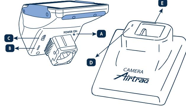
A. Automatic power button: This button is automatically pushed when the A-390 is inserted onto any Airtraq. It can also be pushed manually to turn on the A-390. To turn off the A-390 press the corresponding icon on the menu.
